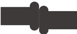
Misalignment. Welding under the condition that the misalignment exceeds 10% of pipe wall thickness while align the two ends.
